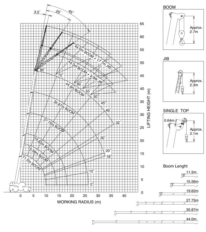
NOTE: The above lifting height and boom angle are based on a straight (unladen) boom, and allowance should be made for boom deflection obtained under laden conditions. The above working range is shown on condition with outriggers fully (7.2m) extended.
